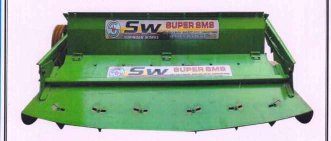
**S W SUPER SMS,** FITTED ON MALKIT 997, SELF- PROPELLED COMBINE HARVESTER
